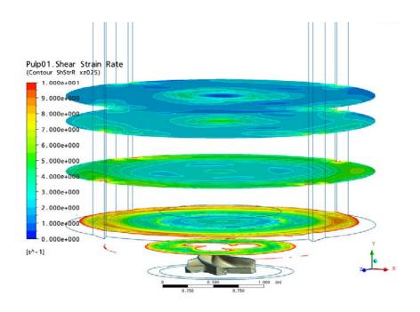
Pulping is most efficiently done by shear force, therefore volume with sufficient shear force can be maximized by rotor and vat design.
